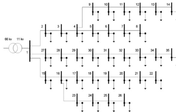
Fig. (3): Single-line diagram of the distributed network
