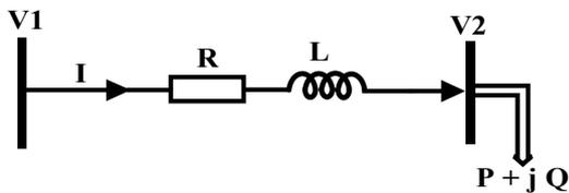
Fig. (1): Equivalent circuit of distribution transformers
