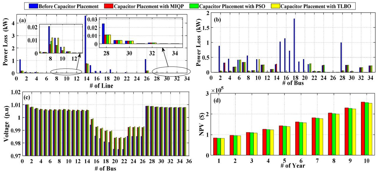
Fig. (7): Results for Industrial Loads: a) Power losses of feeders, b) Power loss of transformer, c) Bus voltages, d) NPV
