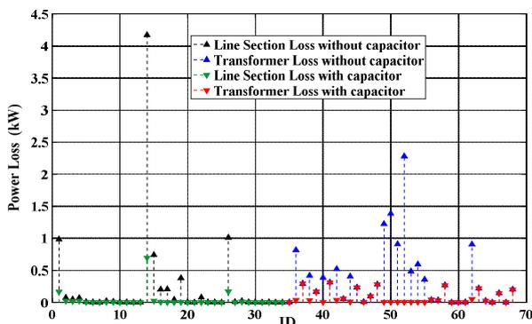
Fig. (5): The power losses components before and after capacitor installation for constant loads
