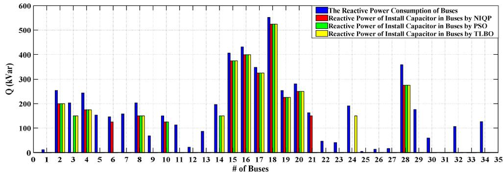
Fig. (4): Reactive power of buses consumption and total capacitor units obtained by MIQP, PSO, and TLBO
