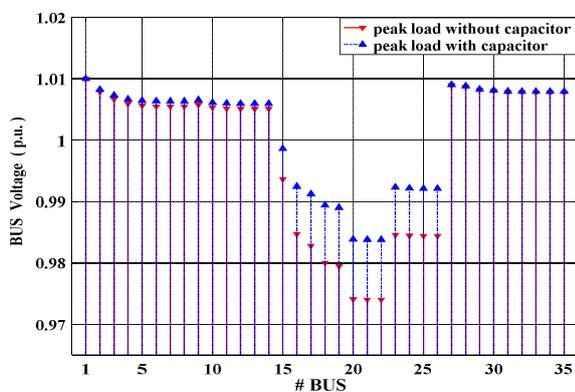
Fig. (6): The magnitude of effective voltages of the busses before and after capacitor installation for constant loads
