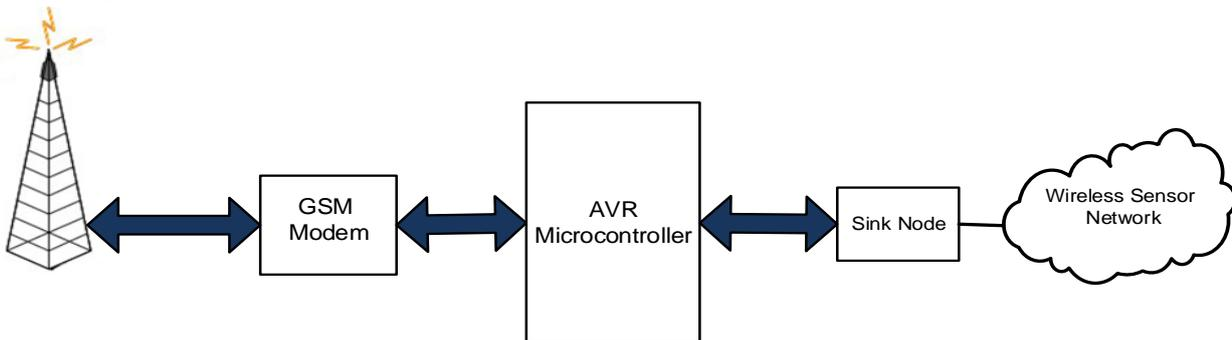
Fig. (8): Hardware in the greenhouse side
