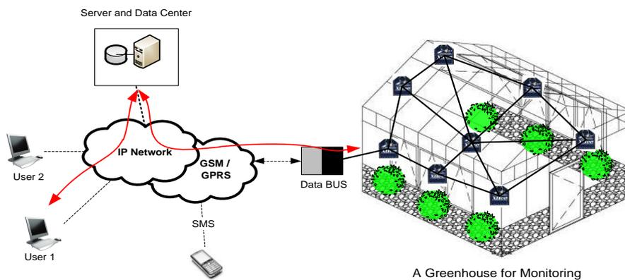
Fig. (1): The proposed structure based on WSN and GSM Link
