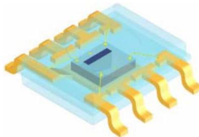
Fig. (3): TSL2550 digital sensor for light intensity
