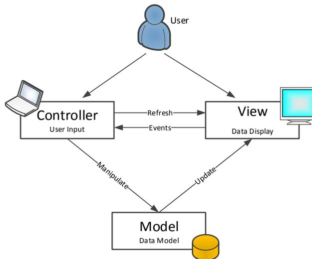
Fig. (10): A typical relationship between the MVC components
