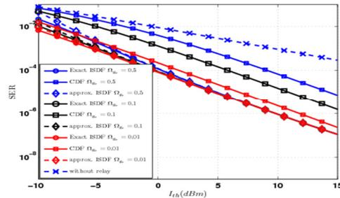
Fig. (4): The SER performance vs. the interference threshold for various  $\Omega_{gr}$ . ( $\Omega_{gs}$  is fixed to 0.01)
