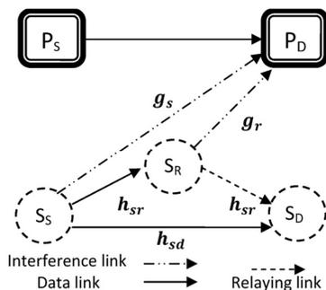
Fig. (1): Protocol of relaying data in two phases in the secondary network
