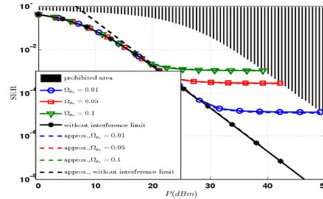
Fig. (3): The SER performance vs.  $P$  for various  $\Omega_{gs}$ . ( $\Omega_{gr}$  is fixed to 0.01)
