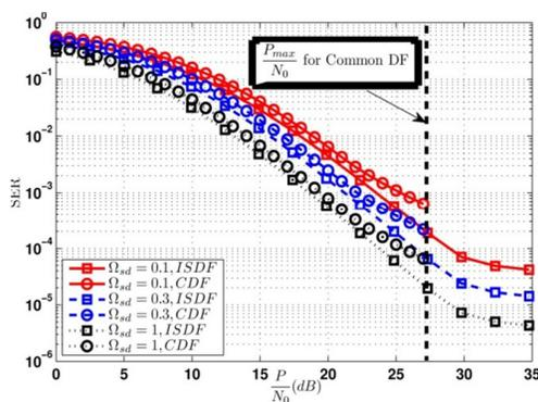
Fig. (5): The SER performance comparison for the ISDF protocol respect to fixed DF for various  $\Omega_{sd}$ . ( $\Omega_{gs} = 0:01; \Omega_{gr} = 0:1$ )
